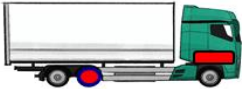
Figure 3-2: Volvo 6x2 fuel cell electric truck as part of the FC-1 vehicle combination for use case 7.2.1
