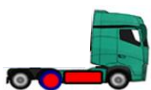
Figure 3-9: Renault 6x2 battery electric tractor as part of the BEV-6 vehicle combination for use cases 7.4.1, 7.4.2 and 7.4.3
