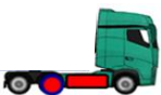
Figure 3-4: Volvo 6x2 battery electric tractor as part of the BEV-2 vehicle combination for use cases 7.2.3
