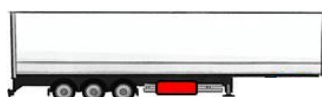
Figure 3-15: battery trailer as part of the BEV-4 and BEV-5 vehicle combination for use case 7.3.1
