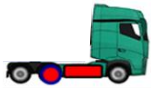
Figure 3-6: Scania 6x2 battery electric tractor as part of the BEV-4 vehicle combination for use cases 7.3.1 and 7.3.3
