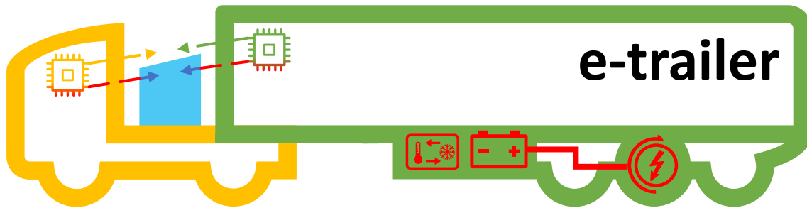
Figure 2-1: Illustration of the main powertrain components of the e-trailer and the interfaces to the prime mover
