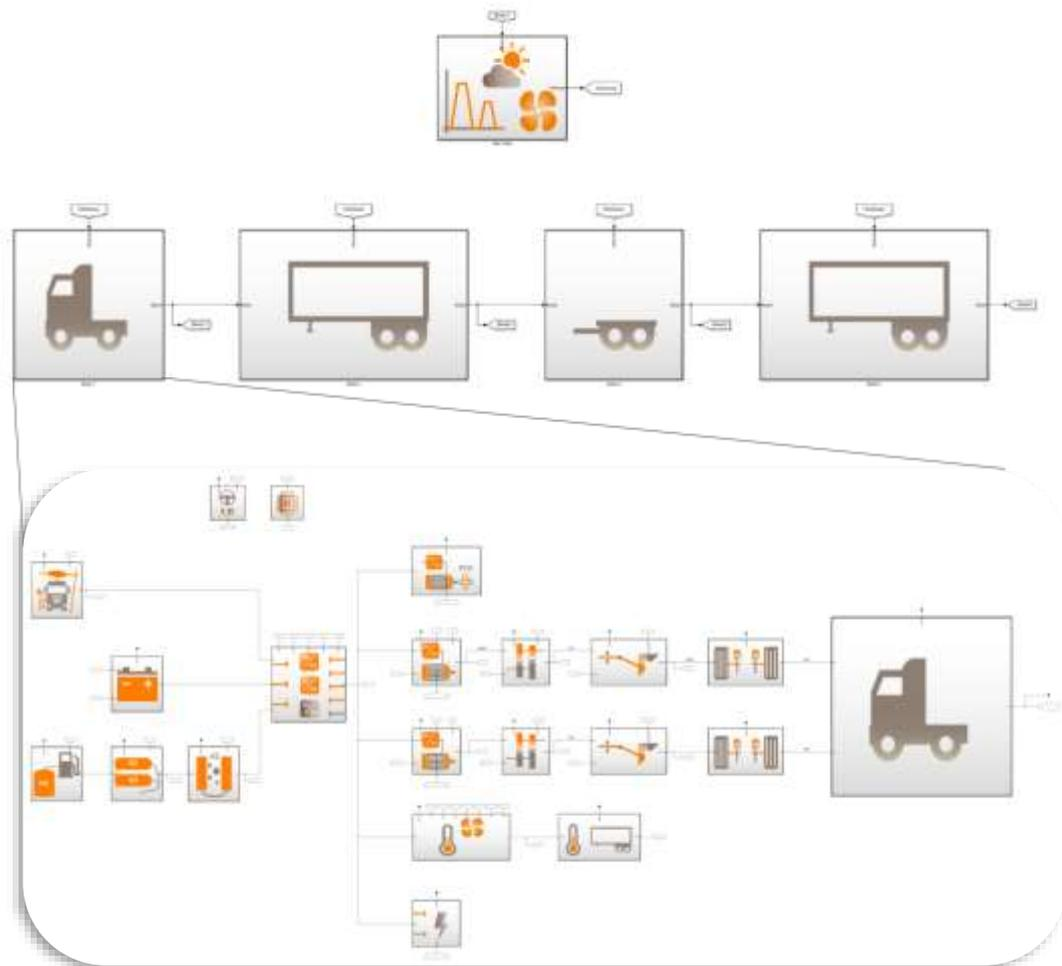
Figure 11. Simulink model of the truck with its subcomponents for each body.
