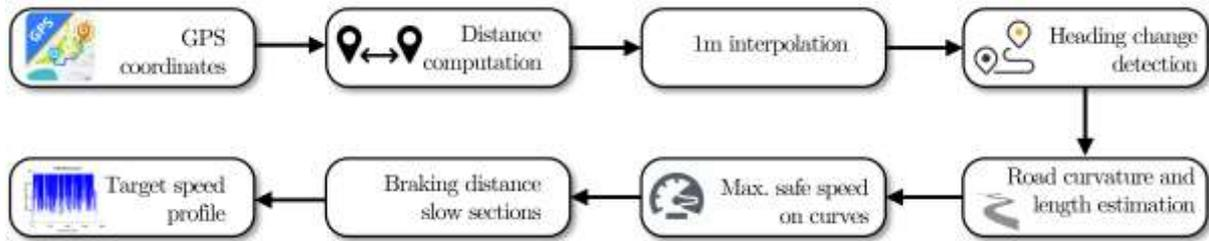
Figure 6. Flowchart for producing the vehicle mission profile of ZEFES use-cases.
