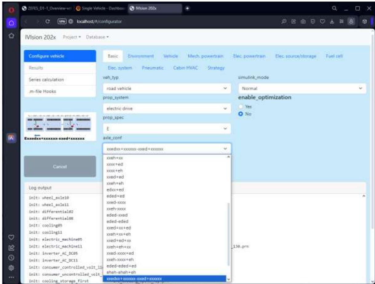
Figure 26. User interface for vehicle configuration.
