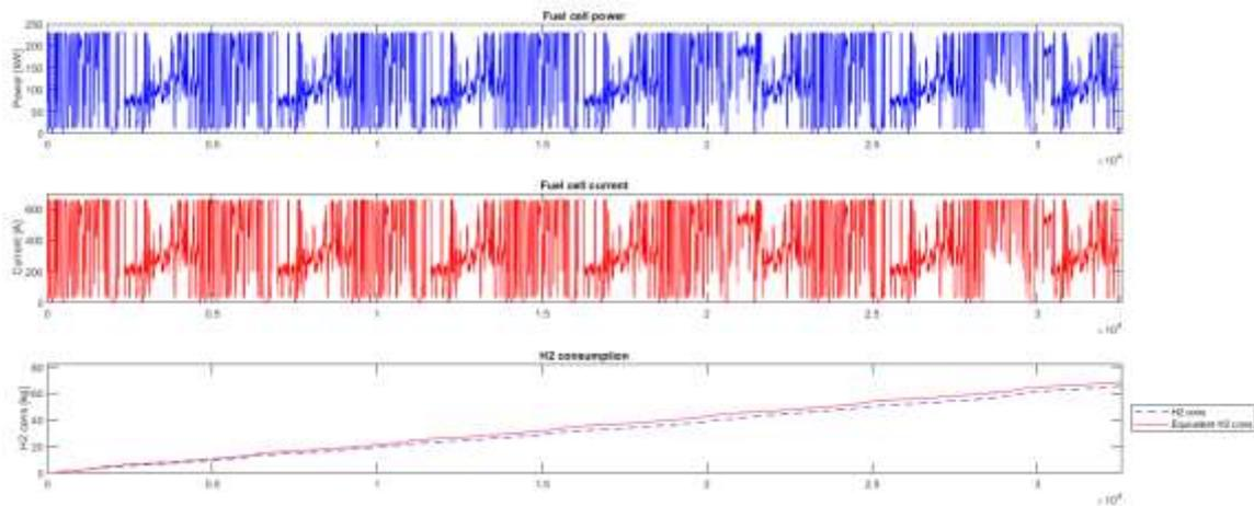
Figure 18. Simulation results for FCEV architecture (initial 13% battery SOC and doubled FC power scale factor, VECTO long haul cycle 750km).
