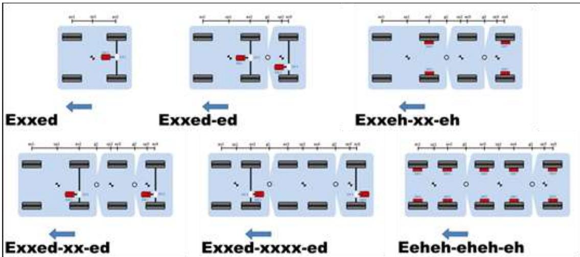
Figure 24. Examples for electric powertrain configurations.
