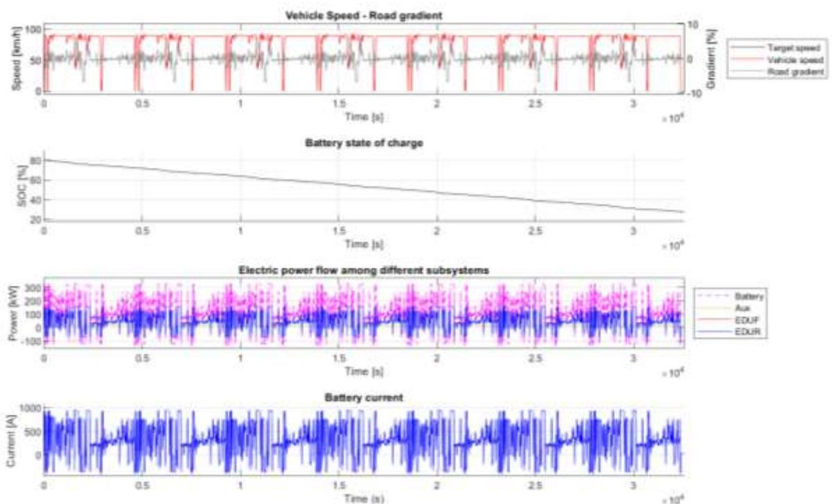
Figure 16. Simulation results for BEV2 architecture (BEV2 initial 80% SOC, VECTO long haul cycle 750km).
