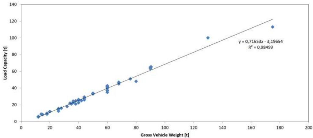
Figure 33. Load capacity as a function of gross vehicle weight.
