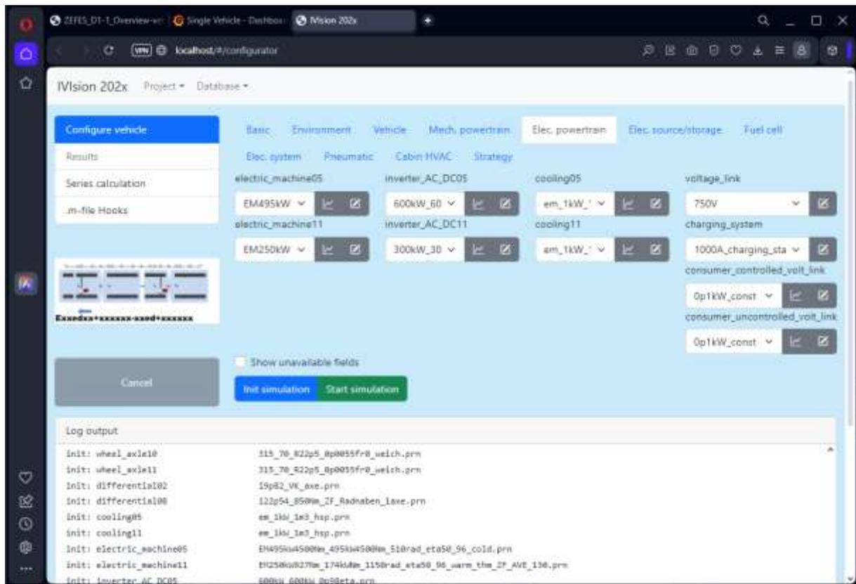
Figure 27. User interface for vehicle configuration.
