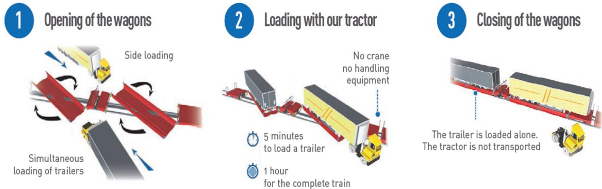
Figure 33. Working mechanism of intermodal train station in Le Boulou.
