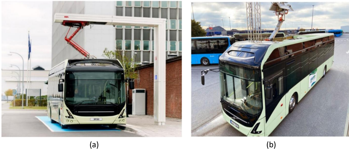
Figure 5 The use case demo with fast charging using pantograph technology in Gothenburg, Sweden. (a) Infrastructure mounted ACD by ABB, (b) Roof mounted ACD
