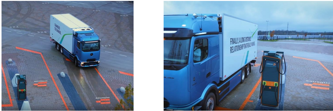
Figure 12 Video demonstration of truck accessing the charging bay [15]
