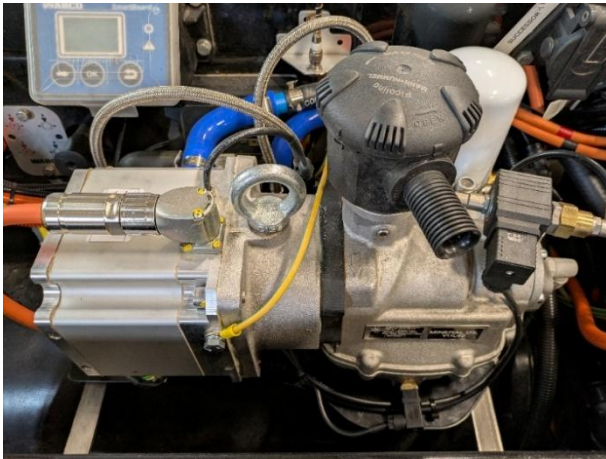
Figure 2-9: Installed MOTEG eAir V60 high-pressure air compressor
