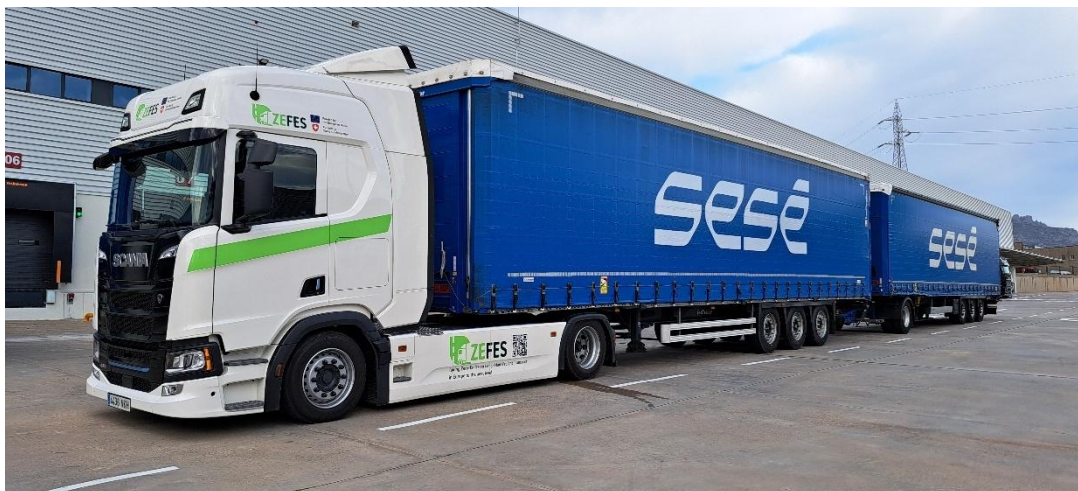
Figure 4: Scania tractor unit in EMS2 vehicle combination with two mega trailers and a standard converter dolly (use case 7.3.4)
